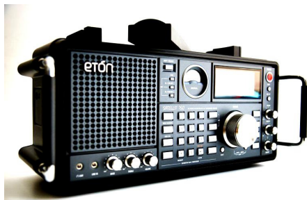
Grundig Satellit 750: World Band Receiver for LW, MW, SW - AM, SSB, FM / FM
