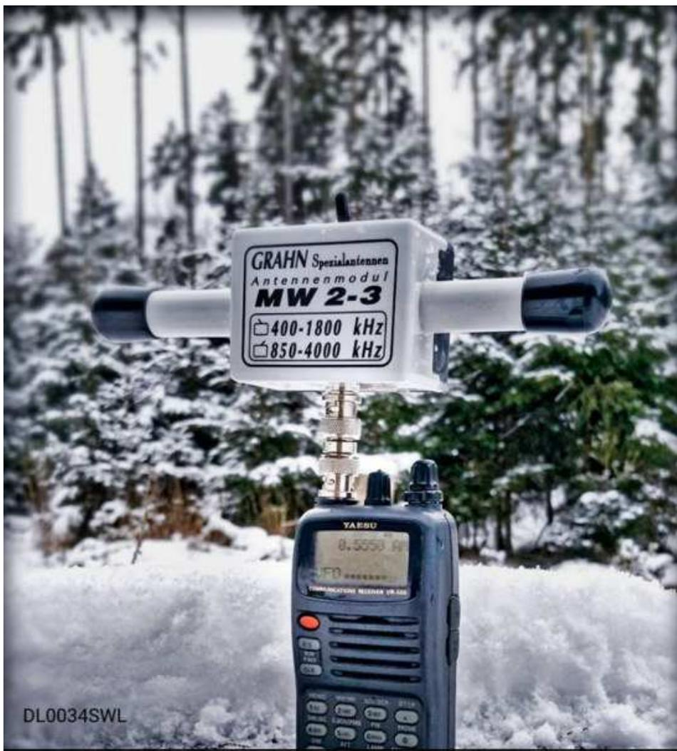
ANTENNAS Modules ferrite VLF-LW-MW
