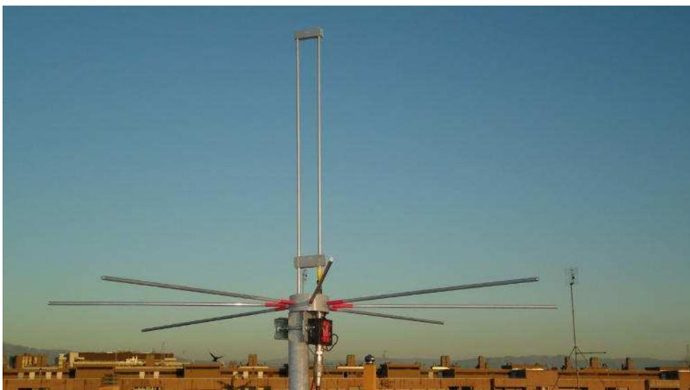
Fig. 5 antenna ground plane
