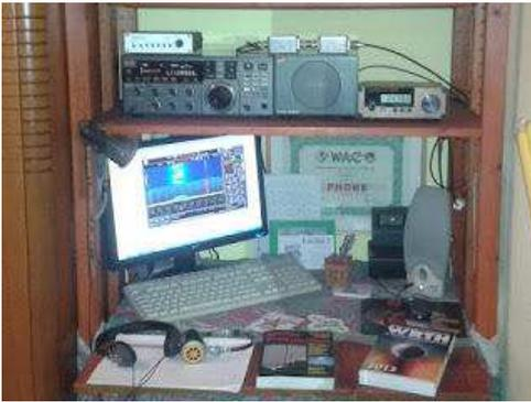
*IK2GFT-SWLI2-1510 Buccinasco SW Milano Italy -JRC 525 NRD-LOWE HF 150-Elad FDM S2 -Antenna LOOP ALA100M- MiniWHIP -Filter PAR Electronics LPF - HPF -Lat. 45.25'.00" Long. 9.7'.00" -Locator grid. Jn 45 Nk-*
