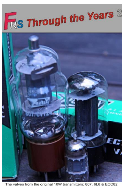
The valves from the original 10W transmitters: 807, 6L6 & ECC82
