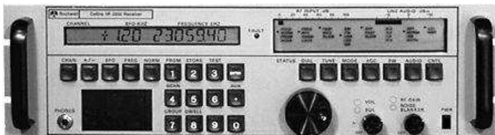
**The Rockwell HF-2050 General Purpose VLF/LF/MF/HF Receiver**
