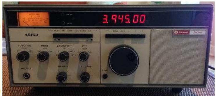
Fully Synthesized in 10 Hz steps. General Coverage 0.2 to 30 MHz Internal Microprocessor Control. Solid-State Modular Construction. SSB/CW and AM Modes. Passband Tuning. Built-in AC/DC Power Supply and Speaker. Digital Frequency Readout. ( **Deriva dal transceiver KWM-380** <http://www.collinsradio.org/cca-collins-historical-archives/the-equipment-of-collins-radio/the-s-word-or-solid-state/kwm-380/> )
