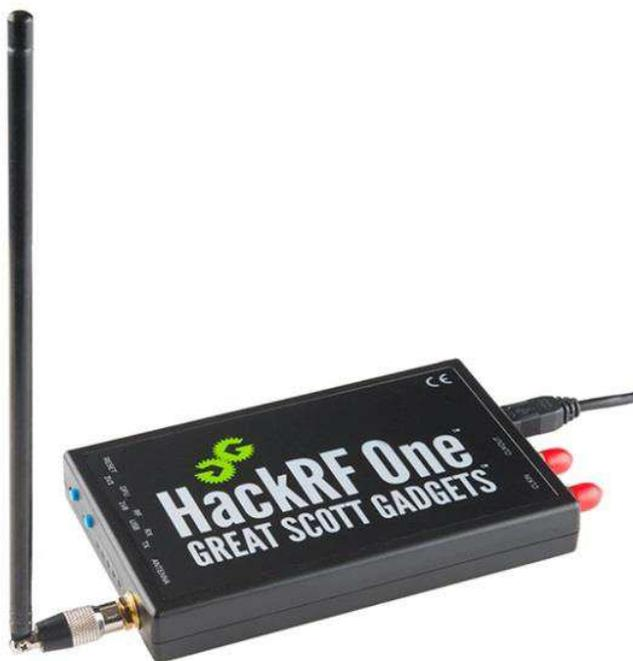
The HackRF is a \$300 USD RX/TX capable software defined radio which has a wide tuning range from almost DC – 6 GHz, and wide bandwidths of up to 20 MHz. It uses an 8-bit ADC so reception quality is not great, but most people buy it for its TX and wide frequency/bandwidth capabilities.
