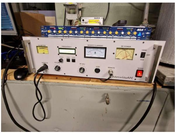
**2 kW Hercules transmitter of which 400 watts is regularly used. (Northern Star Media Services AS)**
