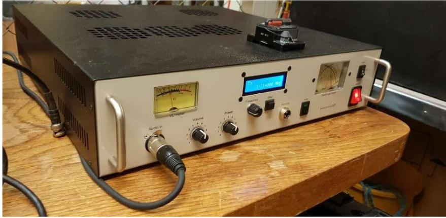
**1kW Hercules transmitter 1314 kHz of which 700 watts is regularly used. (Foreningen Bergen Kringkaster, picture: Northern Star Media Services AS)**
